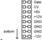
The bottom is the edge of the PC board
